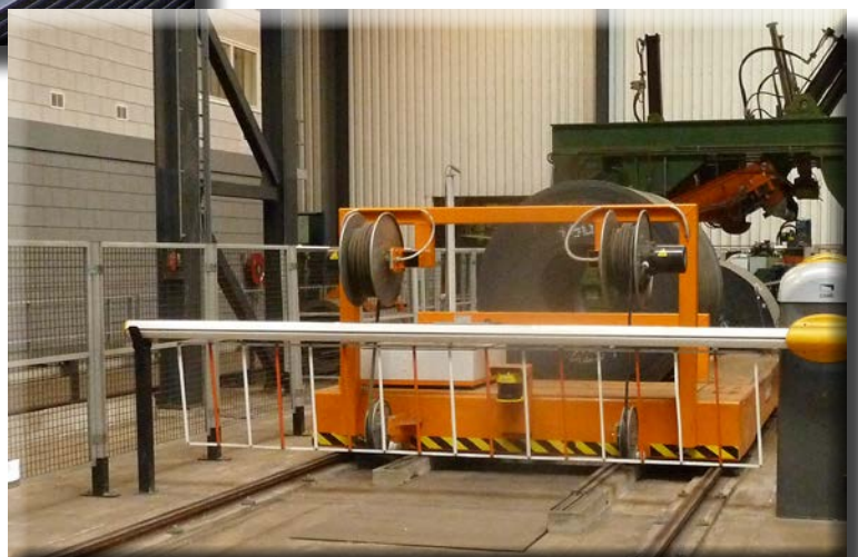
AV40 cable reels for feeding and controlling of a transfer cart and machines
