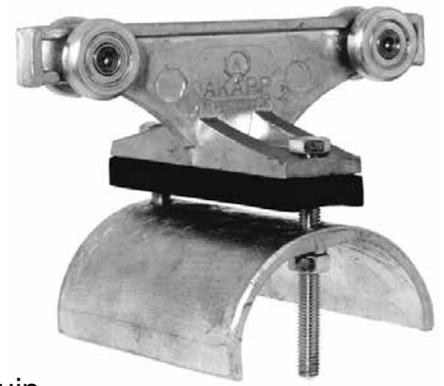
AKAPP aluminium cable trolleys for track profile R300 are especially suited to average sized installations, for both in- and outdoor conditions. The steel wheels are ball beared. The trolleys therefore will roll perfectly smooth through the track profile. The trolleys are equipped with a rubber strip to press against the cable(s).
