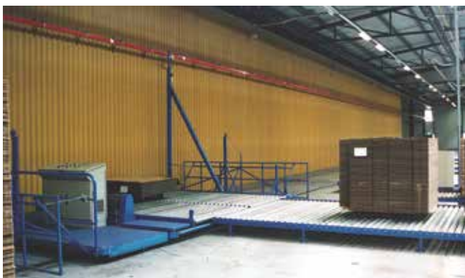
Conductor housing, type RN7 for feed and control of a traverse car in a carton processing plant.
