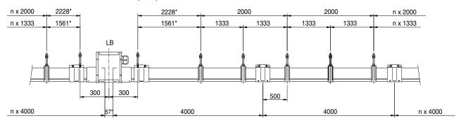
When clamp holder RN-LH is applied: 57 = 0 mm; decrease other dimensions marked with \* by 28 mm
